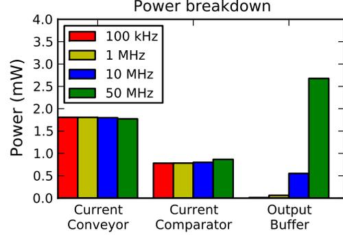
Figure 5. Power breakdown in the 3M2P  $0.5 \mu\text{m}$  process.
