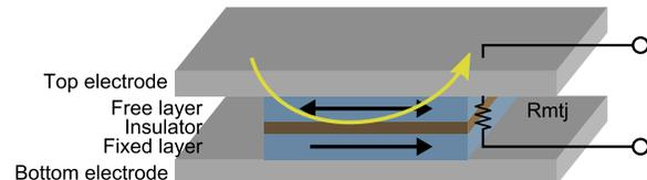
Figure 1. A magnetic tunnel junction (MTJ) device with state information encoded in the magnetic orientation of the free layer. An external magnetic field applied to the free layer sets this state and it is accessed as a resistance ( $R_{mtj}$ ) between the two electrodes.
