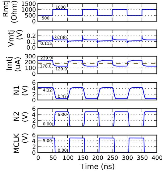
Figure 4. Transient response of the R2V read circuit at 10 MHz frequency.  $R_{mtj}$  is the input resistance,  $V_{mtj}$  is the voltage over  $R_{mtj}$ ,  $I_{mtj}$  is the current through  $R_{mtj}$ ,  $N1$  is the current comparator output,  $N2$  is the first inverter output, and  $MCLK$  is the read circuit output. Threshold current,  $I_{th}$ , is indicated by the dashed line on  $I_{mtj}$ .
