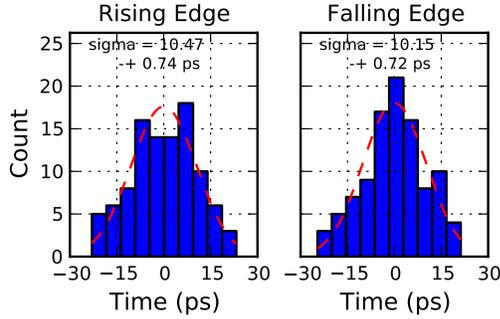
Figure 6. Jitter histogram of the rising/falling edges of MCLK due to noise in the 3M2P 0.5  $\mu\text{m}$  process.
