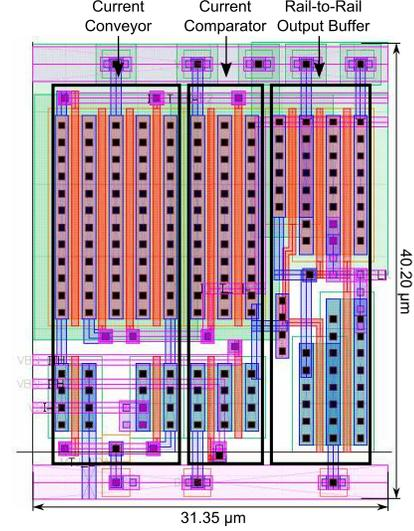
Figure 3. Layout of the R2V read circuit in the 3M2P 0.5  $\mu\text{m}$  process. The sub-circuits highlighted in black boxes are (left) current conveyor, (middle) current comparator, and (right) rail-to-rail output buffer.
