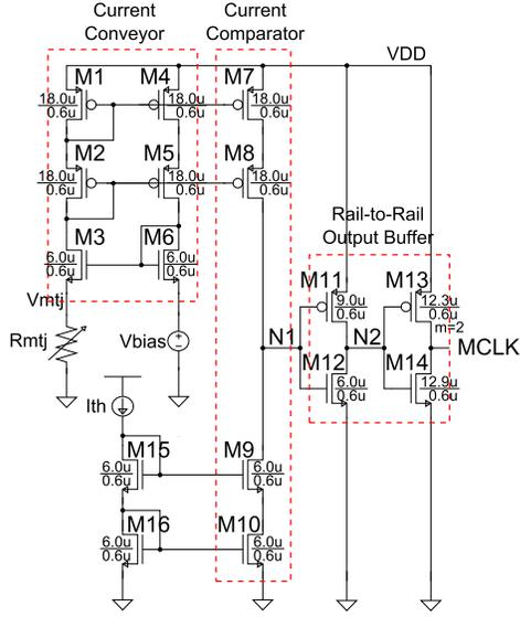
Figure 2. Resistance-to-voltage (R2V) read circuit (3M2P 0.5  $\mu\text{m}$  process).
